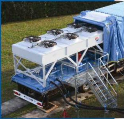
The Güntner Vario FLAT S-GFH dry cooler has special dimensions and fits perfectly on the container. To ensure safe transport, it was also stiffened and the copper piping was reinforced.
