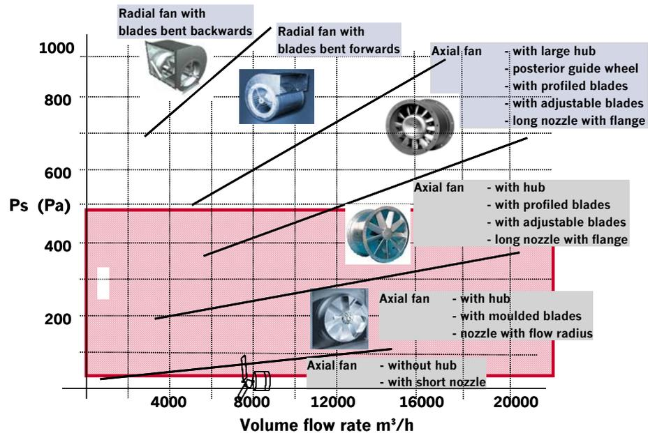
Fans with high delivery volumes are mainly needed in refrigeration and air conditioning engineering for pressure differences between 50 and 200 Pa.
