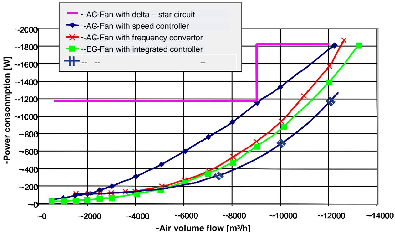
The greatest motor losses occur at reduced speed when using voltage control with a phase cut controller, a transformer or with delta / star switching.
