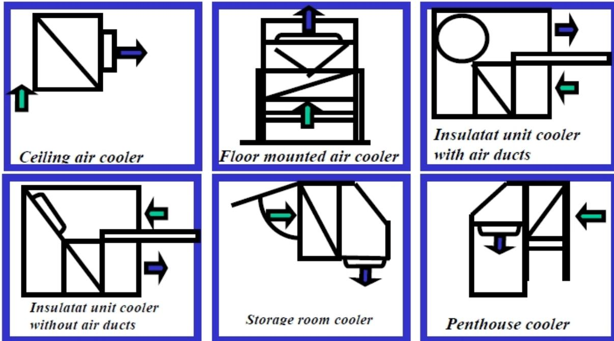
Figure 1. Six types of air coolers
