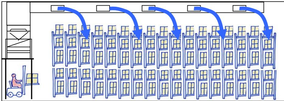
**Figure 3. Floor-mounted air cooler with air ducts**
