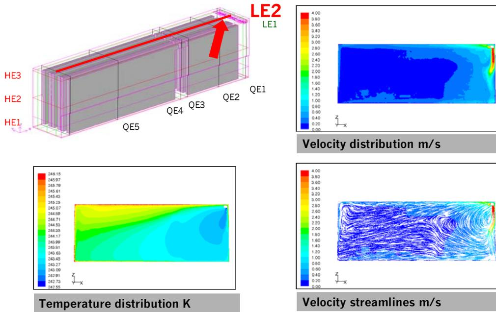
The graphic representation of the air convection shows that only a part of the air flows back to the cooler after about 20 m [65 ft] of room length. (Figure 12) Most of the air flows all the way down the length of the room to the opposite outer wall,
