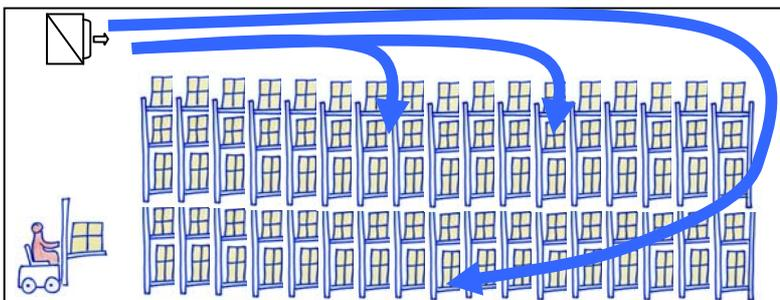
Figure 2. Ceiling air cooler with horizontal air flow
