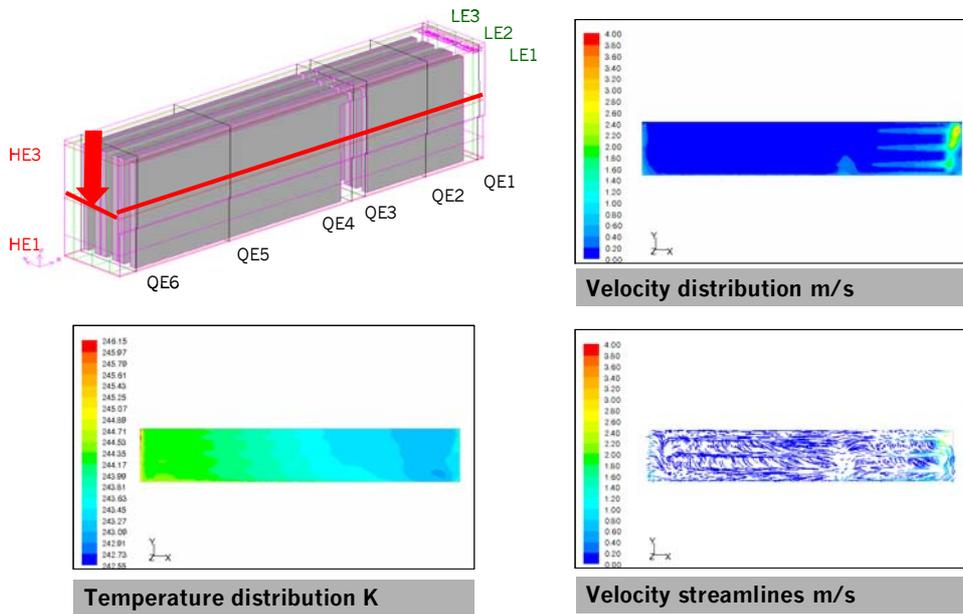
The air speed in the section reduces after approximately 20 m [65 ft]. (Figure 11) The cold air flows down the section to the end of the room. At the outer walls, warmer air convects upward. The temperature difference over the length of the room is about 1.4 K [2.5°F] in this section.
