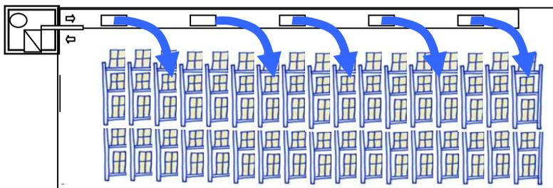
**Figure 4. Insulated unit air cooler with air ducts**
