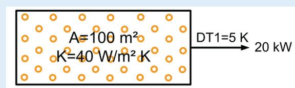
Fig. 8: Highly efficient evaporator with larger surface
