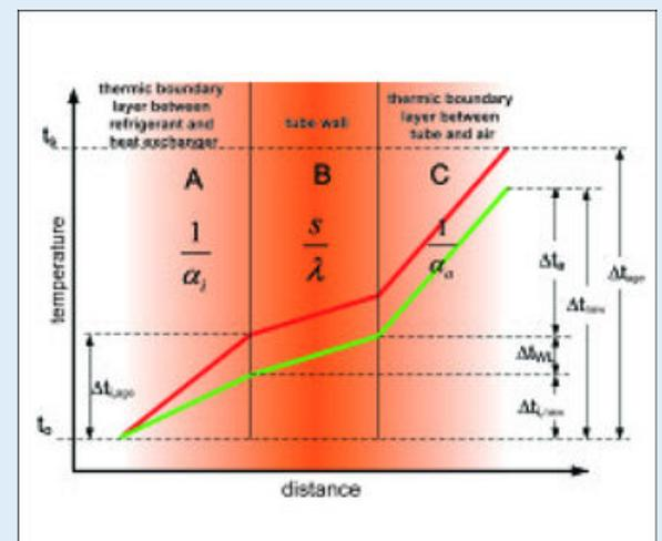
Fig. 2: Temperature pattern through a refrigerant carrying tube with increased internal heat transfer
