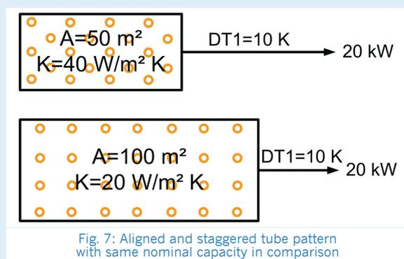
Fig. 7: Aligned and staggered tube pattern with same nominal capacity in comparison
