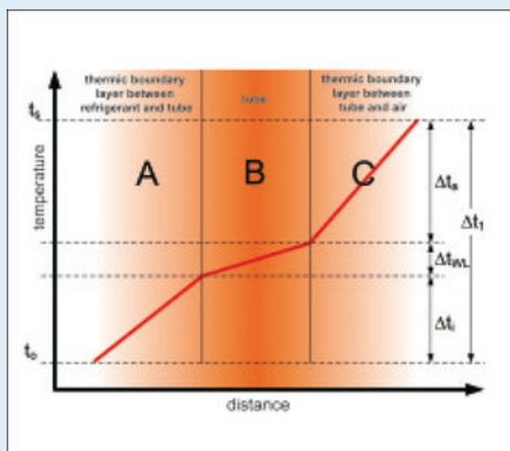
Fig. 1: Temperature pattern through the wall of a refrigerant-carrying tube
