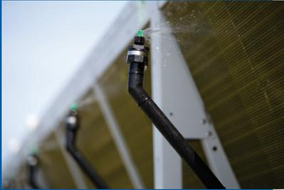
▲ Spraying can be controlled individually for all sections.
